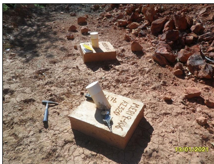
Figure 12.1 Cement Monument for RC Hole MER19-005 and MER19-006
