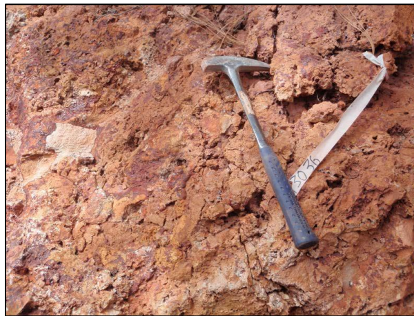
Figure taken from April, 2019, Mercedes Property Technical Report. *Assays returned 1.2 m grading 2.07 g/t gold and 58 g/t silver.
