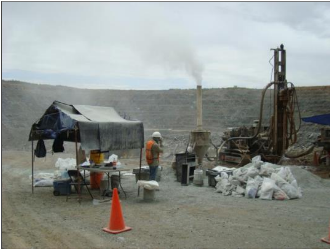
Figure 11.2 Reverse Circulation Sample Collection
