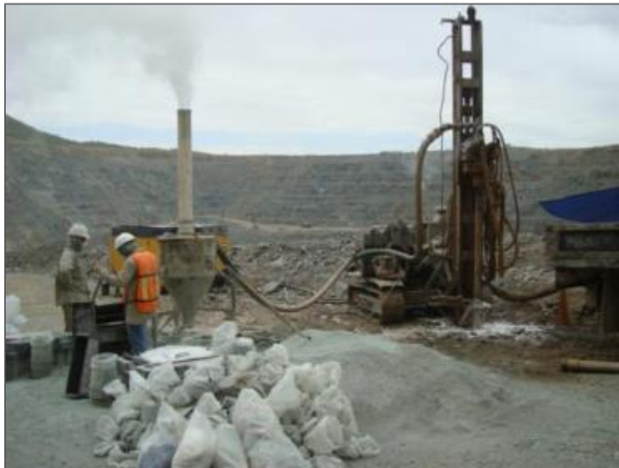
Figure 10.1 RC Drilling in the San Francisco Pit in July, 2011
