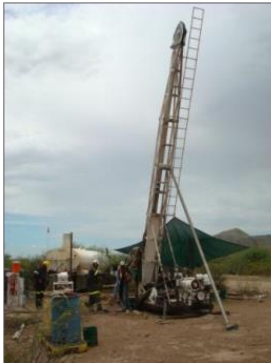
Figure 10.2 Diamond Drill Rig Set-Up on a Drill Hole Southeast of the San Francisco Pit
